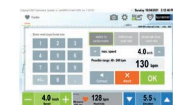
Cardio mode allows target heart rate in combination with maximum speed range definition for controlling the physical load by means of a combination of speed & elevation.
