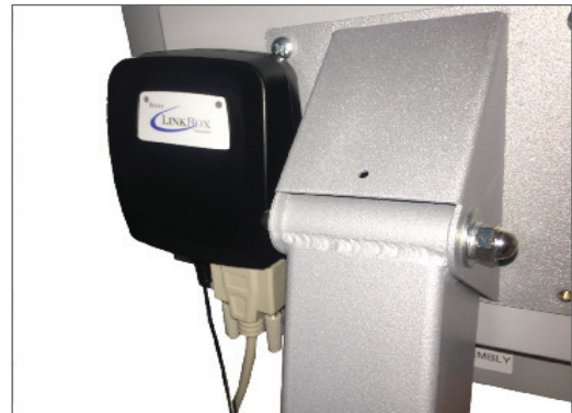
LinkBox wireless communication connected to the Biodex Balance System SD sends and receives signals from the TactileBelt.
